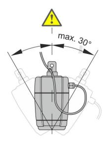
DOL 53 must be mounted vertically with the sensor pointing down;  $\pm 30^{\circ}$  at a location with low vibration and, as far as possible, stable temperatures.
